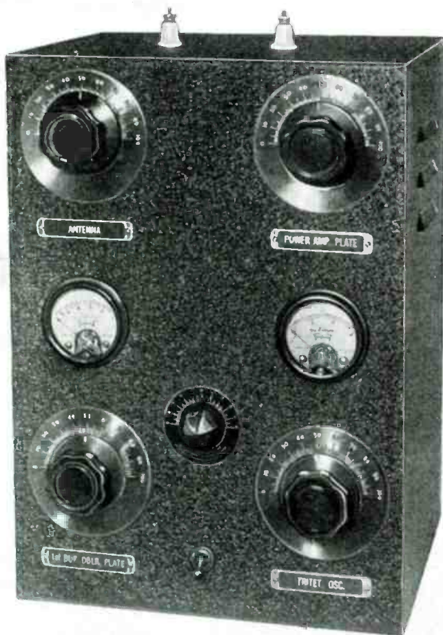
Front and rear views of this very compact 35-watt crystal-controlled Transmitter.
